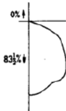
Porcelain-enameled ventilated standard dome with incandescent lamp
