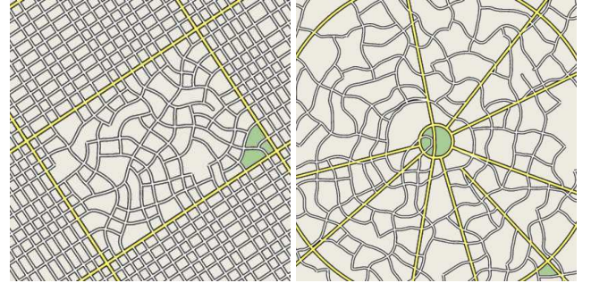
Figure 8: This figure shows a regular major road grid (left) and a radial major road pattern (right) over slightly curved minor roads.
