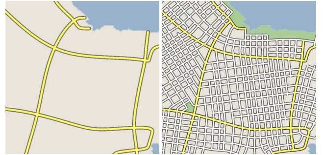
Figure 11: This figure shows a minor road network (right) generated based on the major road network (left)
