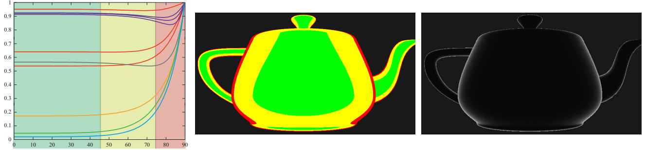
Figure 25: On the left, we can see the Fresnel graph from Figure 24 with overlaid colors for three zones based on the angle between the smooth surface normal and the view or light direction. Green for the zone ( 0^\circ to 45^\circ ) where reflectance is almost constant, yellow for the zone ( 45^\circ to 75^\circ ) where reflectance changes gradually, and red for the zone ( 75^\circ to 90^\circ ) where reflectance goes rapidly to 1. In the center image, these zones are visualized on a 3D object for the angle between \mathbf{n} and \mathbf{v} (which is the relevant angle for Fresnel reflectance in the case of an optically flat surface). On the right we can see the Fresnel reflectance of glass (the green curve in Figure 24) visualized as color on the same object.
