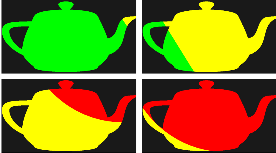
Figure 26: This figure shows the Fresnel zones for the \mathbf{h} vector, using the same approach as for the \mathbf{n} vector in Figure 25. Since the \mathbf{h} vector depends on the light direction \mathbf{l} as well as the view direction \mathbf{v} , the figure contains four images—each for a different light direction. We can see that for certain light angles, the entire object may be in the yellow or even the red zone. As we will see in Figure 27, this is somewhat misleading.
