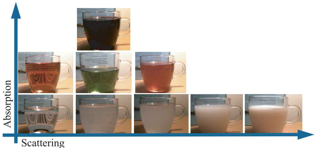
Figure 11: Media with varying amounts of light absorption and scattering. The appearance depends on both properties; for example, a white appearance (lower right) is the result of high scattering combined with low absorption.
